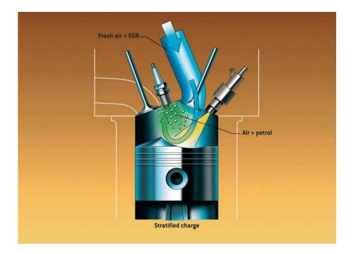
The principle of the stratified charge engine is to deliver a mixture that is sufficiently rich for combustion in the immediate vicinity of the spark plug and in the remainder of the cylinder, a very lean mixture that is so low in fuel that it could not be used in a traditional engine. On an engine with stratified charge, the delivered power is no longer controlled by the quantity of admitted air, but by the quantity of petrol injected, as with a diesel engine.
