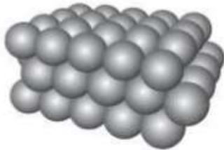
The 3-D arrangement of atoms in a typical metal
