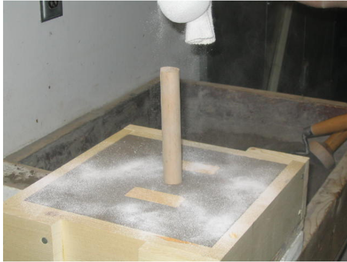
Figure 7 Applying parting Dust
