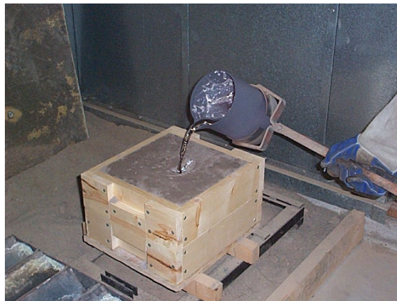
Figure 17 Pouring into the Mold
