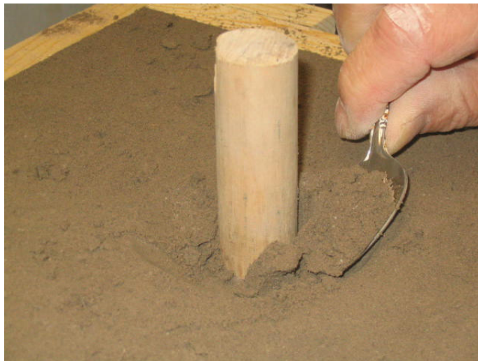
Figure 8 Cutting the Funnel Around the Sprue Pin
