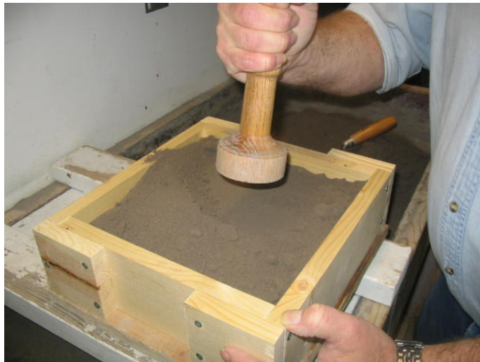
Figure 4 Ramming the Sand
