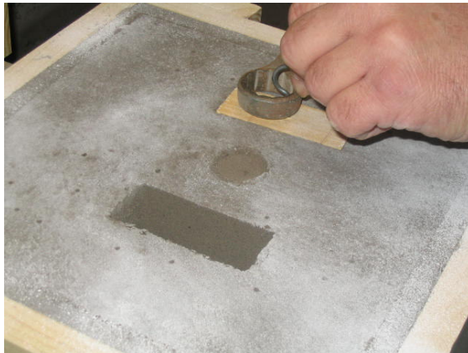
Figure 10 Rapping the Pattern
