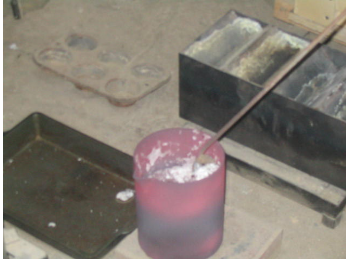
Figure 16 Skimming the Dross
