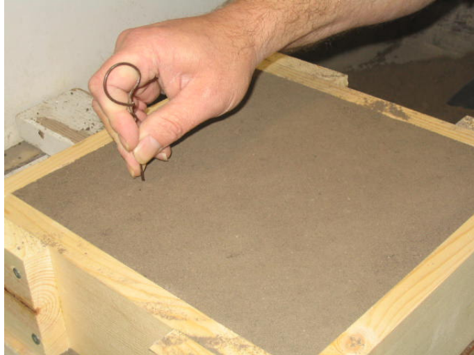
Figure 5 Venting the Sand
