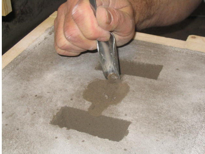
Figure 11 Cutting the Gates
