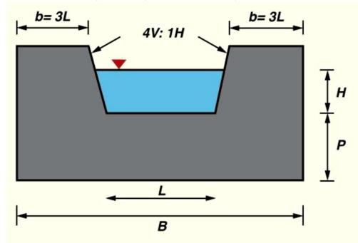
• Discharge for a trapezoidal Weir is calculated as follows:
