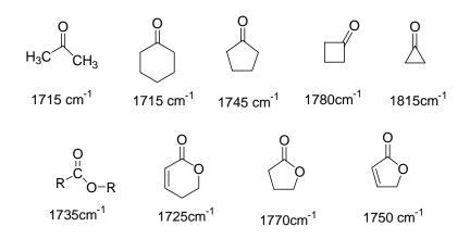
Figure 28 : C=O stretching frequencies in various compounds
