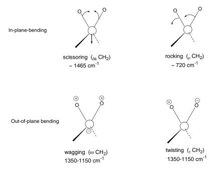
*Figure 14:* Vibrational modes of a  $CH_2$  group. [ $\oplus$  and  $\ominus$  indicate movement above and below the plane of page]
