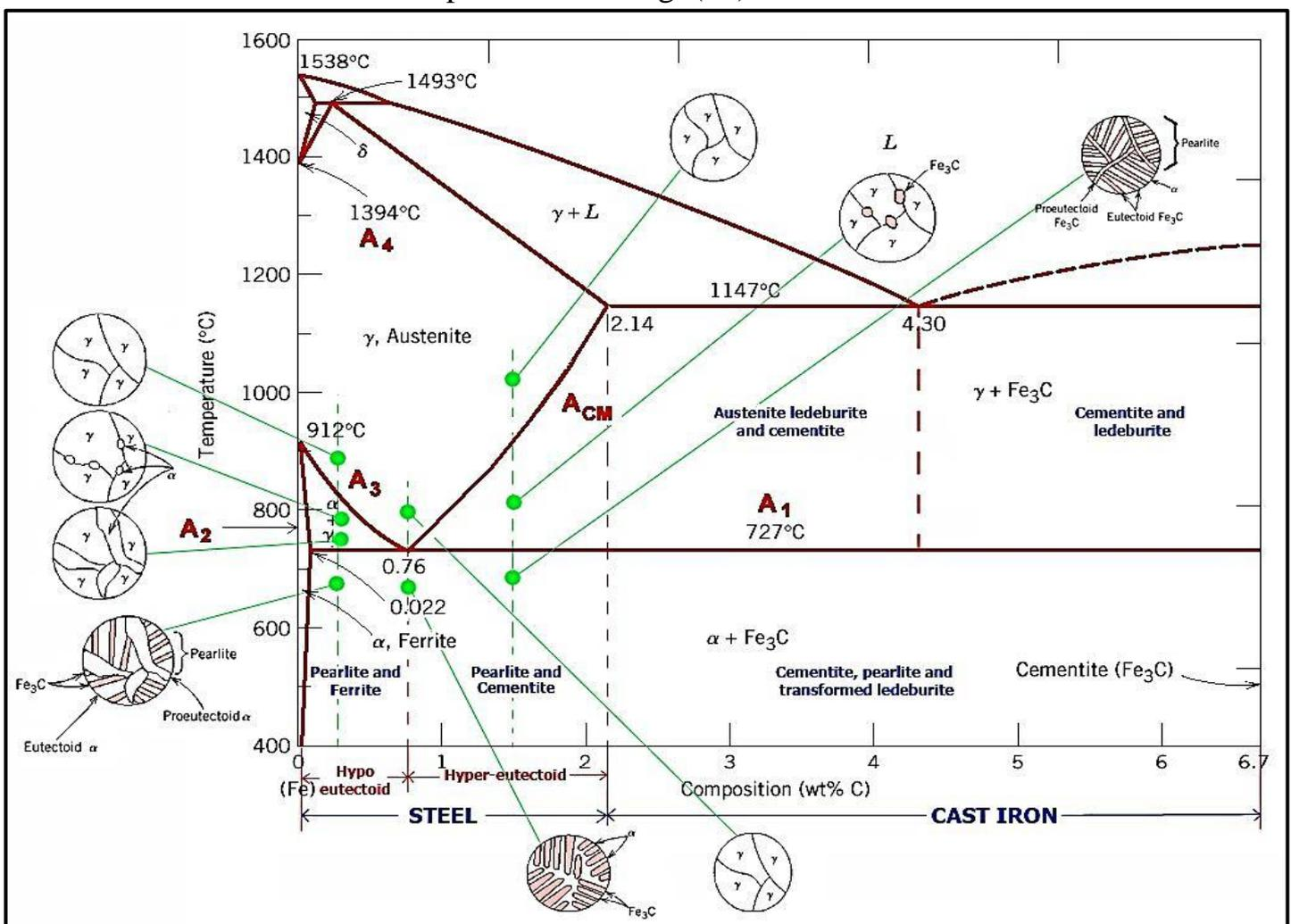
Fig.(25) Microstructure development in Fe-Fe<sub>3</sub>C phase diagram up to 2.06% C.
