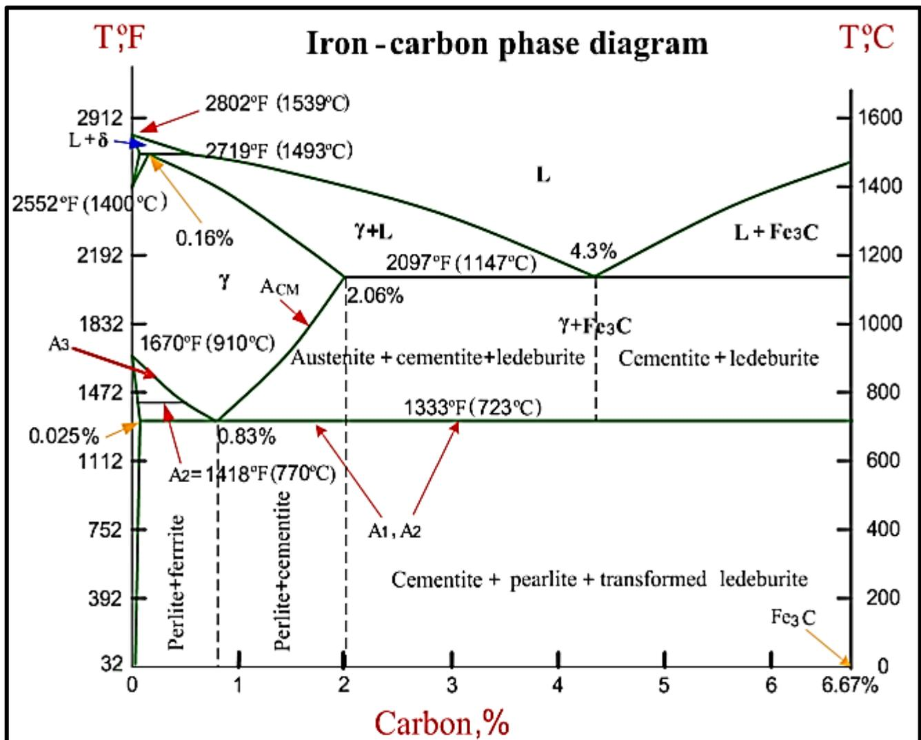
Fig.(24) A portion of the iron–carbon phase diagram which called the Fe–Fe<sub>3</sub>C phase diagram
