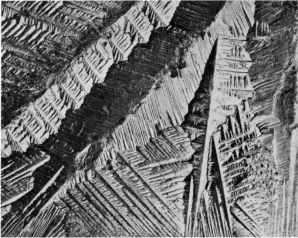
Fig. 6 A Dendrites on the surface of an ingot of antimony. Antimony is one of the few metals which expand during solidification. Hence the growing dendrites were raised clear of the remaining liquid so that their growth could not be completed.
