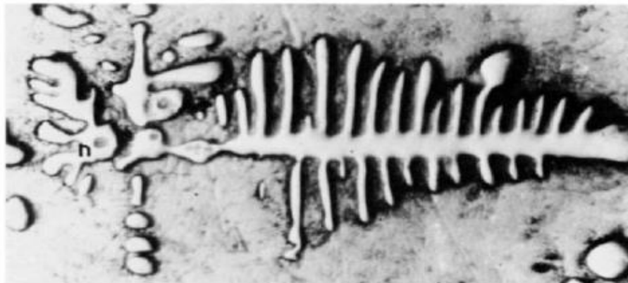
Fig. 3 Dendritic growth. This iron dendrite grew from a nucleus at 'n' in a molten mixture of iron and copper. After all the available iron had been used up the dendrite ceased to grow, and the molten copper solidified as the matrix in which the iron dendrite remains embedded. (In fact the iron dendrite will contain a little dissolved copper—in 'solid solution'—whilst the copper matrix will contain a very small amount of dissolved iron), x 300.
