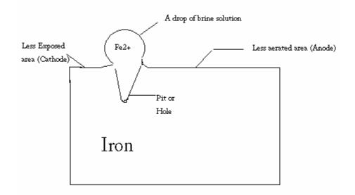
At anode: Fe is oxidized to Fe2+ and releases electrons.
