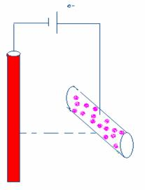
In Impressed-current cathodic protection, electrons are supplied from an external cell so that the object itself becomes cathodic and is not oxidized.
