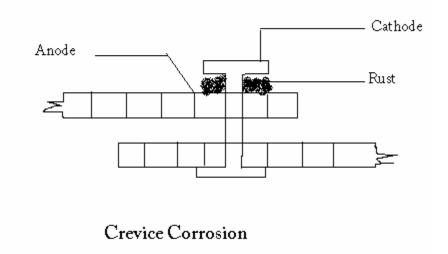
Bolts, nuts, rivets, joints are examples for this type of corrosion.
