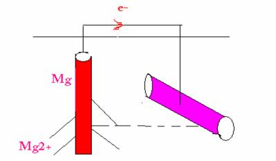
In cathodic protection, an anode of a more strongly reducing metal is sacrificed to maintain the integrity of the protected object (eg., a pipeline, bridge, ship hull or boat).
