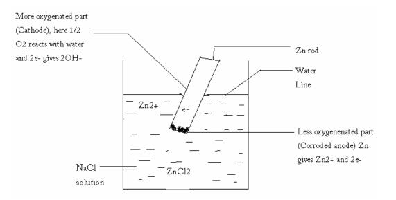
At anode: Corrosion occurs (less aerated)  $M \longrightarrow M^{2+} + 2e^{-1}$
