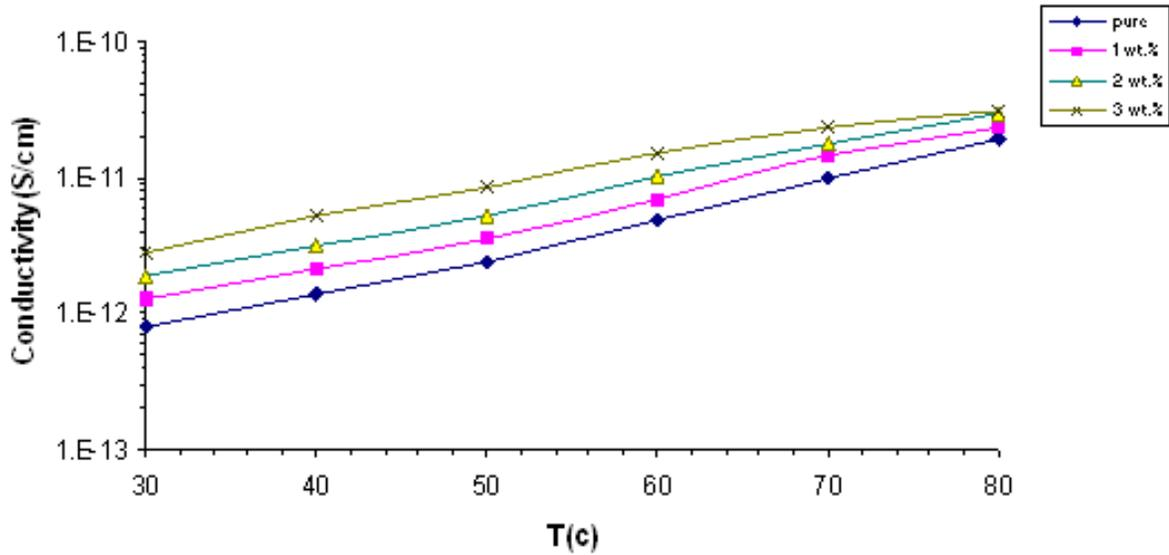
Figure(3) shows the relationship between the  $\ln(\text{conductivity})$  and inverted absolute temperature of the PVA- CaO composites, using equation(2) was calculate activation energy it can be seen that there are high values of activation energy these high values are attributed to the existence of free ions in the polymer. By adding low concentrations of calcium oxide, the values of the activation energy are decreasing for PVA- CaO composites as a result of the impact of space charge [2].
