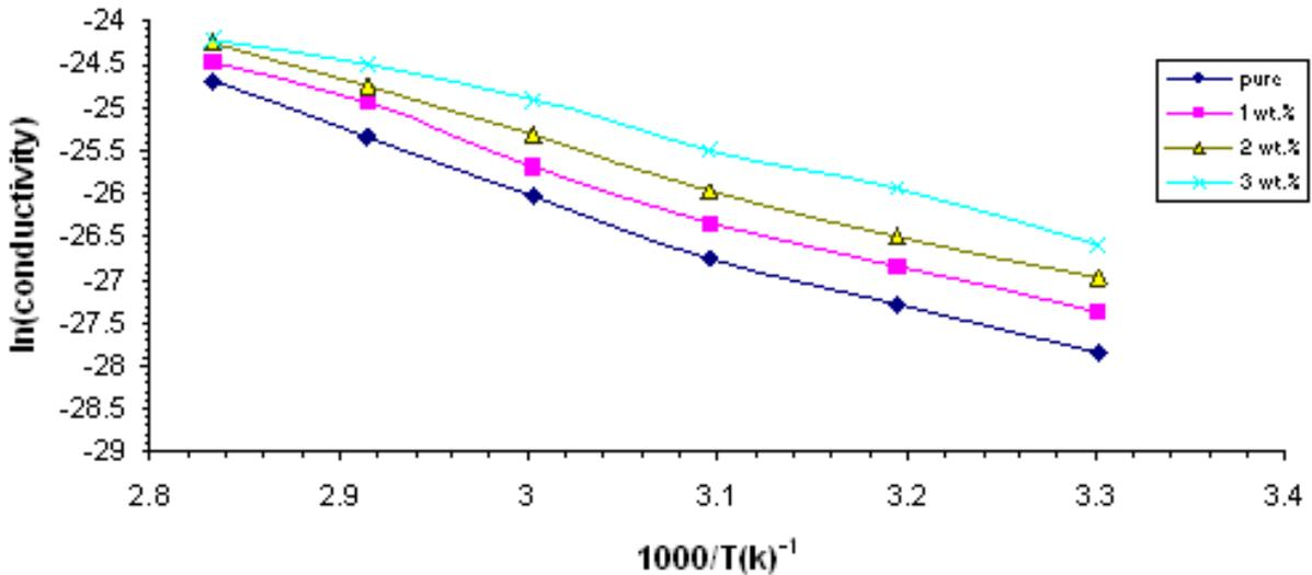
The addition of low concentrations creates local energy levels in the forbidden energy gap which act as traps for charge carriers, which move by hopping among these levels. By increasing the calcium oxide concentrations, the activation energy decreases as a result of the increase of local centres [6], as shown in figure(4) .
