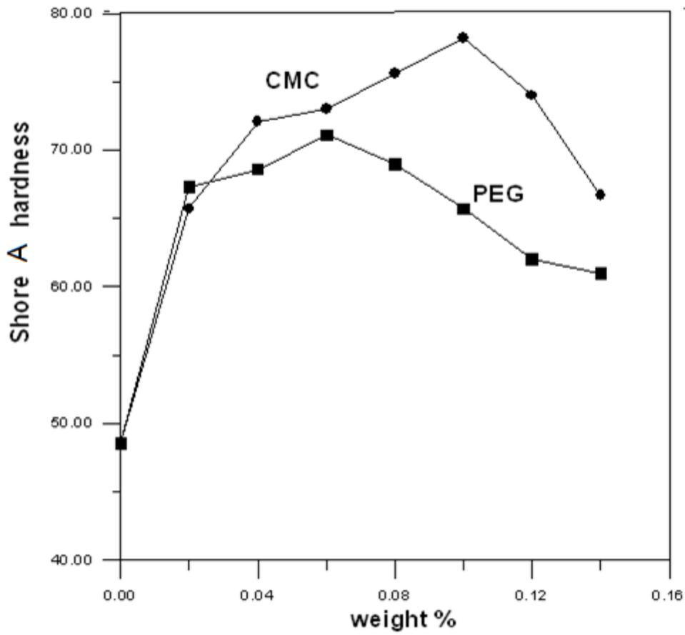
**Fig. (2): relationship between Shore A hardness and the weight fractions of CMC and PEG4000.**
