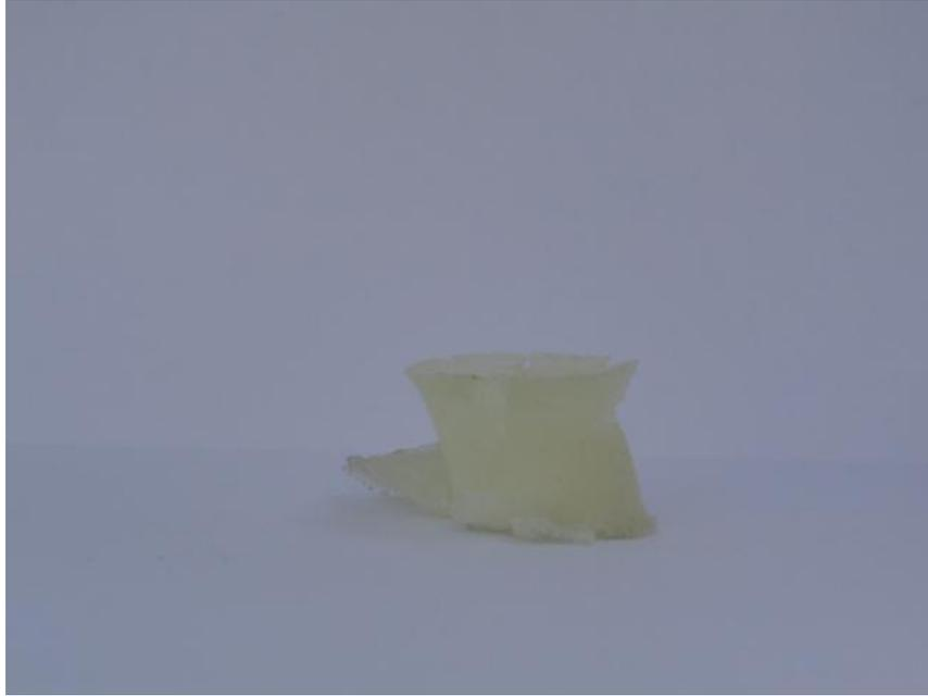
**Fig.(5): the shape of failure of unreinforced epoxy specimen after compression test.**
