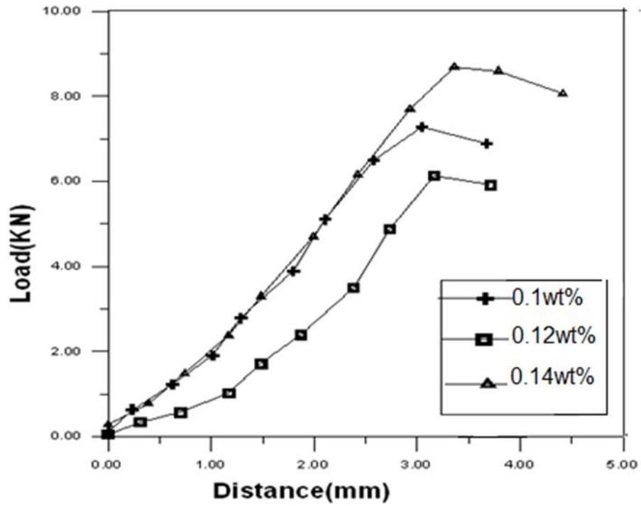
**Fig.(8): data of compression test for epoxy specimens reinforced with PEG (0.1-0.14) wt %**
