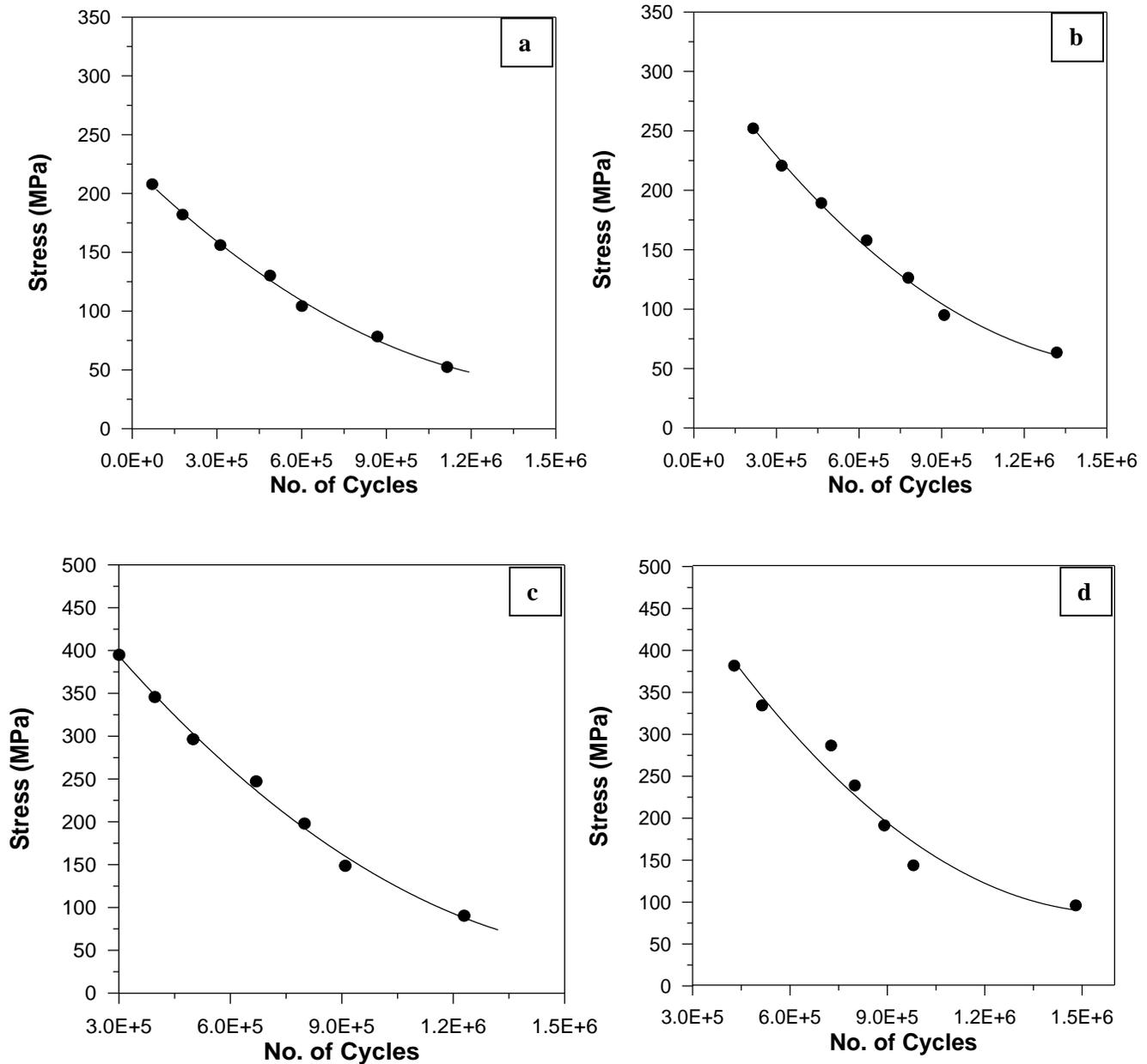
Figure (8). The relation between stress and No. of cycle to failure for carbon reinforced composite: a) 1 layer (0°), b) 2 layers (0°/90°), c) 3 layers (0°/90°/0°), d) 4 layers (0°/45°/-45°/90°)
