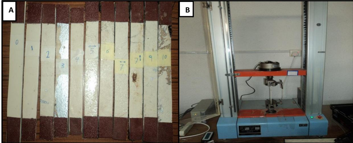
Figure (5): (a) Experimental tensile Specimen, (ASTM D3039), (b) Tensile testing machine
