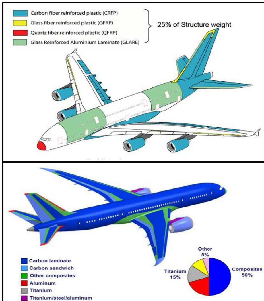
Figure (1) Composite Materials Applications in Commercial Aircraft [3]
