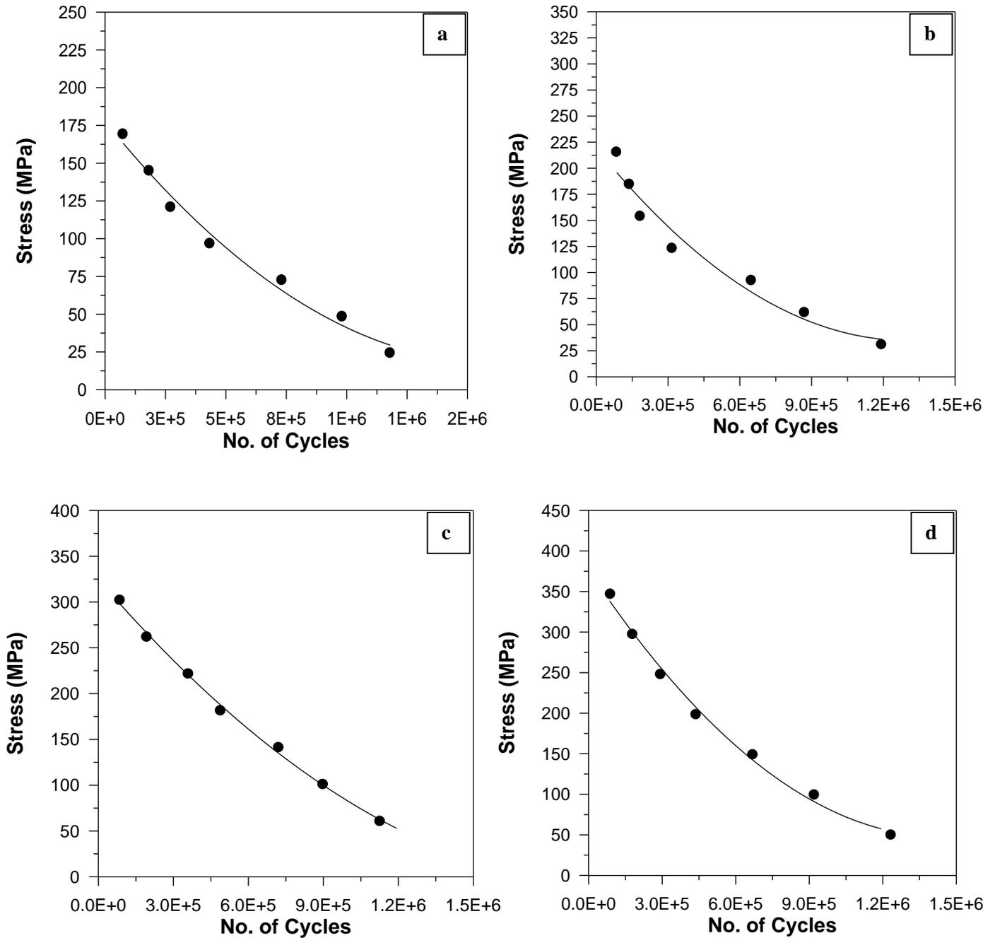
Figure (7). The relation between stress and No. of cycle to failure for glass reinforced composite: a) 1 layer, b) 2 layers, c) 3 layers, d) 4 layers.
