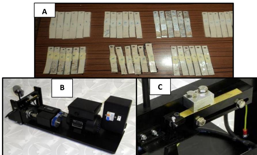
Figure (6): (a) Experimental fatigue specimen, (b) fatigue testing machine and (c) Fixation of specimen
