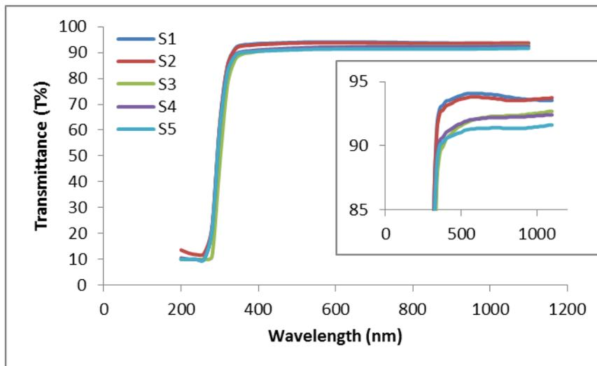
Fig.(7): Transmittance spectra of Al and Al-Ni-Cr nanofilms measured at thickness of 8 nm.
