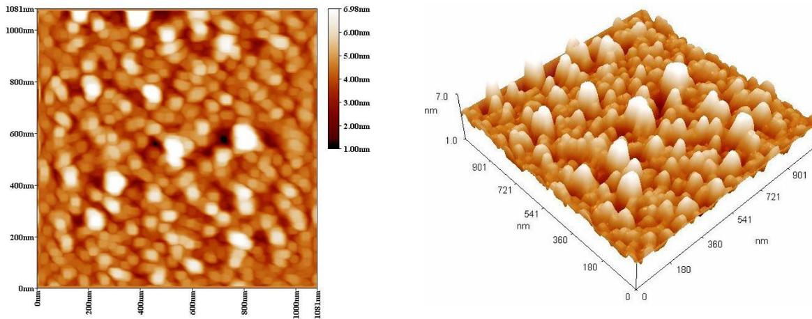
Fig.(5): AFM images for nanostructured film evaporated from S<sub>4</sub> sample, (a) 2D, and (b) 3D.
