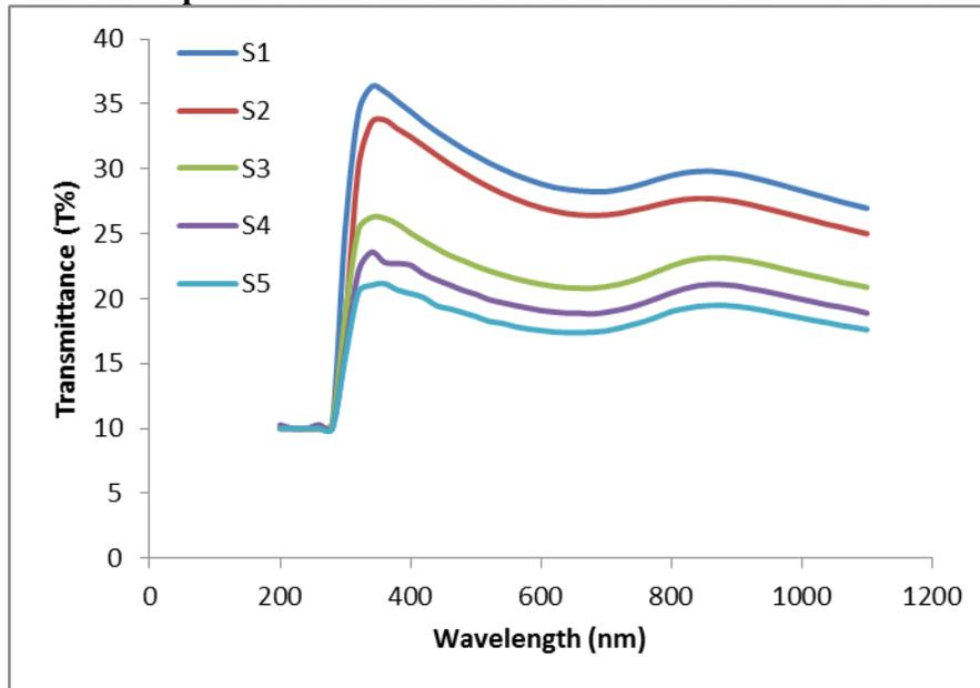
Fig.(9): Transmittance spectra of Al and Al-Ni-Cr nanofilms measured at thickness of 25 nm.
