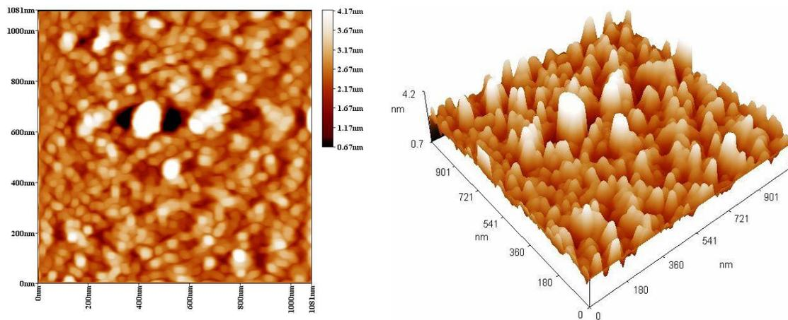
Fig.(4): AFM images for nanostructured film evaporated from S<sub>3</sub> sample, (a) 2D, and (b) 3D.
