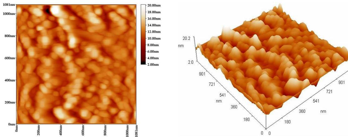
Fig.(2): AFM images for nanostructured film evaporated from  $S_1$  sample, (a) 2D, and (b) 3D.
