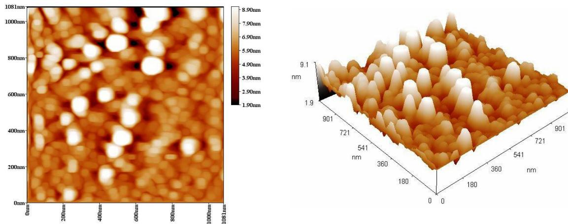
Fig.(3): AFM images for nanostructured film evaporated from  $S_2$  sample, (a) 2D, and (b) 3D.
