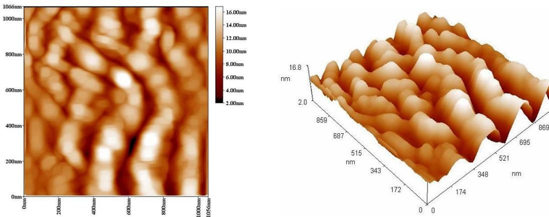
Fig.(6): AFM images for nanostructured film evaporated from S<sub>5</sub> sample, (a) 2D, and (b) 3D
