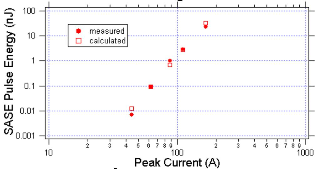
Gain = 10<sup>5</sup> for the two-meter undulator
