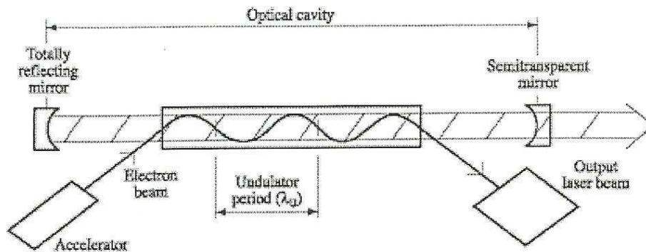
Fig. 2 Typical FEL layout (single passage)
