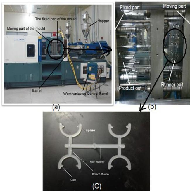
Fig.(2): (a) injection machine JMI/SPI-150 used to produce cylinder part (b) mold of cylinder part (c) Runner waste
