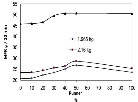
Fig. (12) : MFR behavior with the runner percentage increasing for different loads of second size at 230 °C
