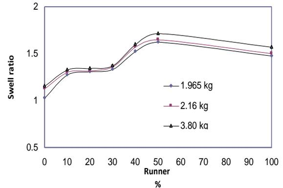
Fig. (8) : swelling ratio behavior with runner percentage increasing for different loads of the first size at 230 °C
