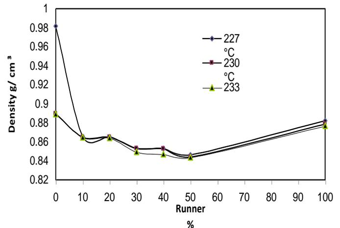
**Fig. (15): density behavior with the runner percentage for different temperatures of second size at load 2.16 kg**
