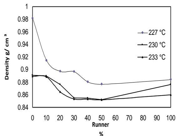
Fig. (9) :density behavior with runner percentage increasing for different temperatures of the first size at load 2.16 kg
