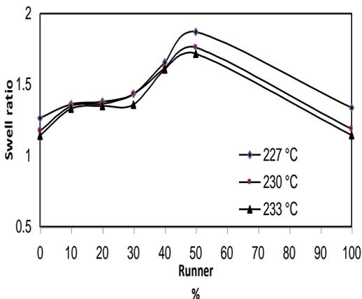
**Fig. (13) : Swelling Ratio Behavior with the runner percentage for different temperatures of second size at load 2.16 kg**
