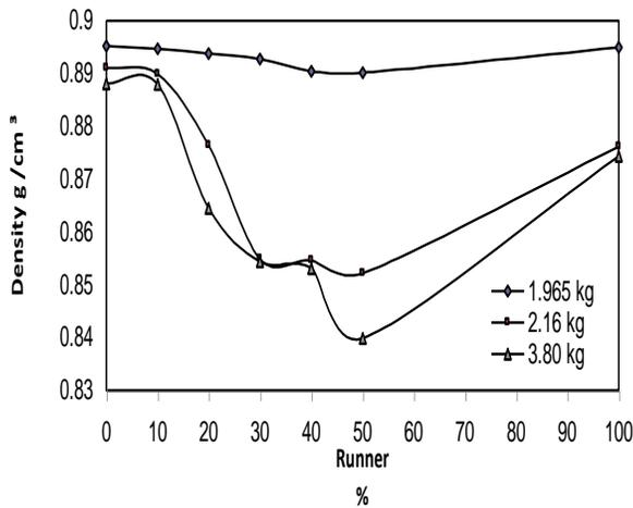
Fig. (10): Density behavior with runner percentage increasing for different loads of the first size at 230 °C
