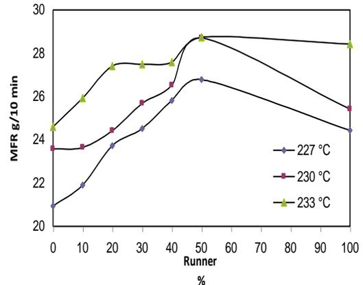
Figure (11): MFR behavior with the runner percentage increasing for different temperatures of second size at load 2.16 kg
