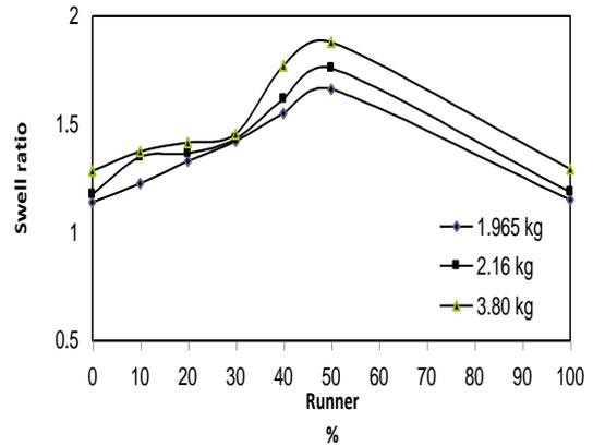
**Fig. (14) : swelling ratio behavior with the runner percentage for different loads of second size at 230 °C**
