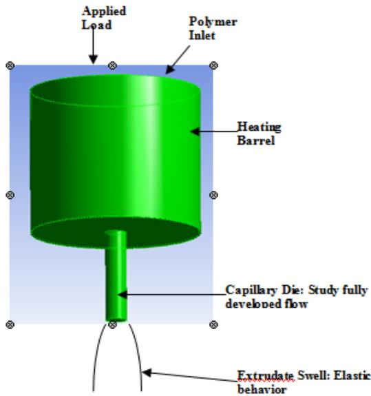
Fig.(3): Schematic of Melt Indexer
