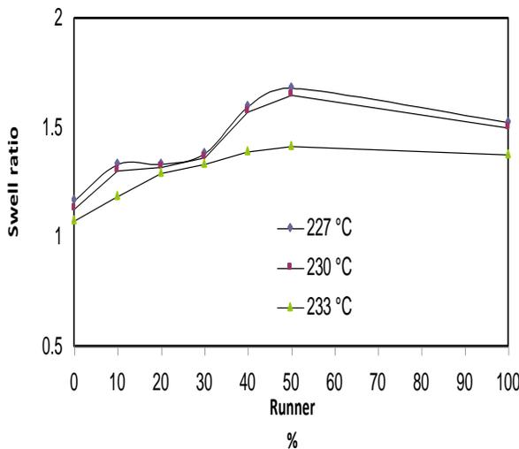
Fig. (7): Swelling ratio effect with runner percentage increasing of different temperature for the first size at load 2.16 kg
