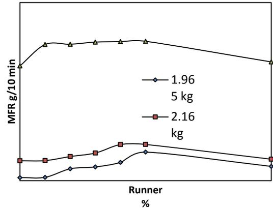
**Fig. (6) : MFR behavior with Runner percentage increasing for different load of the first size at 230**
