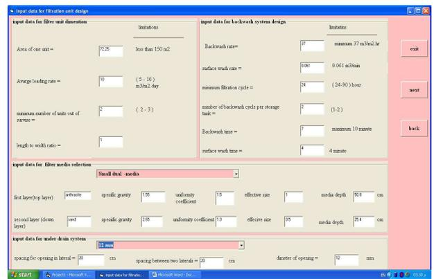
Fig. (8) Input data needed to design filtration unit
