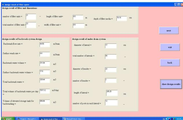
Fig. (7) Module for design filtration unit
