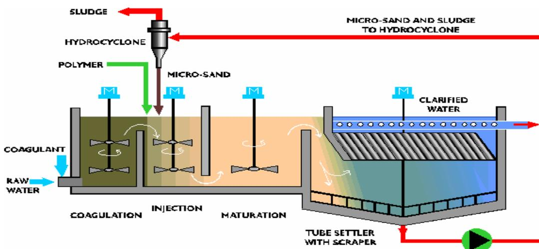
Figure (1) Actiflo Process Flow Diagram
