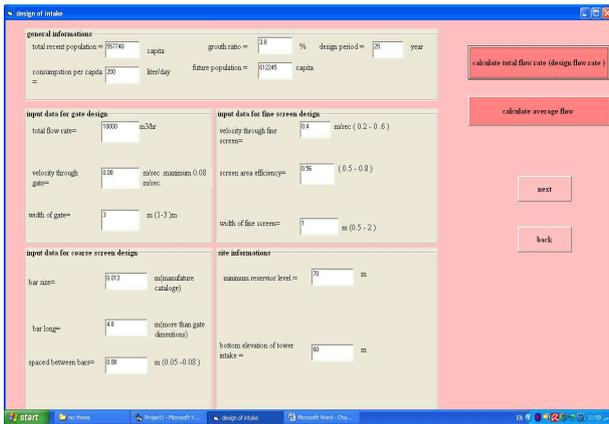
Fig.(3) General Information necessary for design the Actiflo Water Treatment Plant
