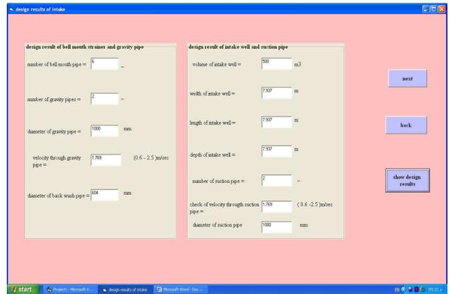
Fig. (4): Module for design intake
