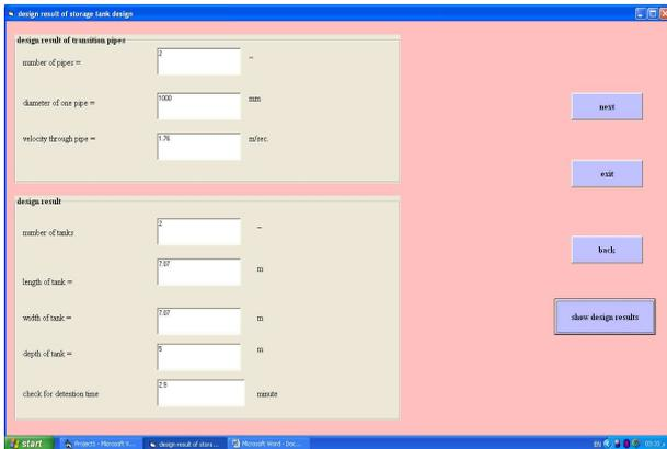
Fig. (5) Module for design transition pipes and Storage unit
