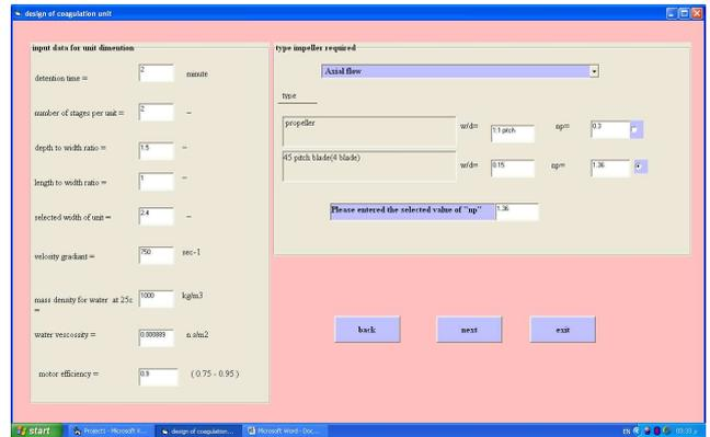
Fig. (6) Input data needed to design coagulation unit
