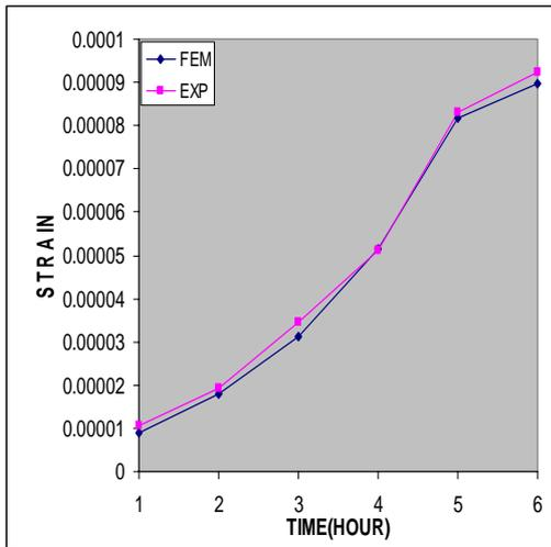
Figure (6) the experimental and theoretical creep results (in x & y direction) of pure low density polyethylene.
