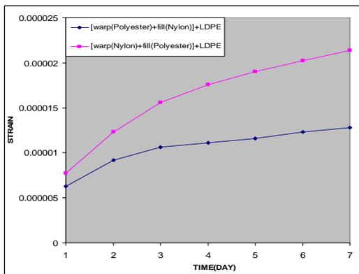
Figure (8) biaxial creep of composite material from hybrid woven fabrics (Nylon with Polyester) fibers and pure low density polyethylene (LDPE) under (450N).
