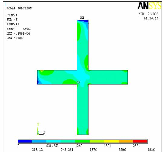
Figures (5-A,B,C,D,E,F) numerical results for biaxial creep of pure low density Polyethylene
