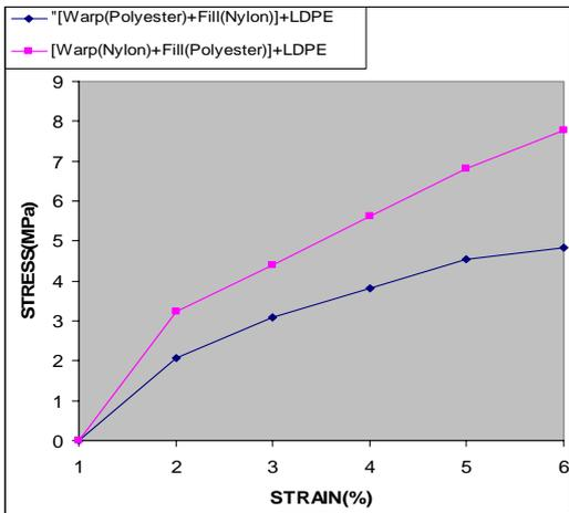
Figure (7) Tensile strength of composite material from (Hybrid woven fabrics (Nylon, Polyester) fibers and pure low density polyethylene(LDPE).
