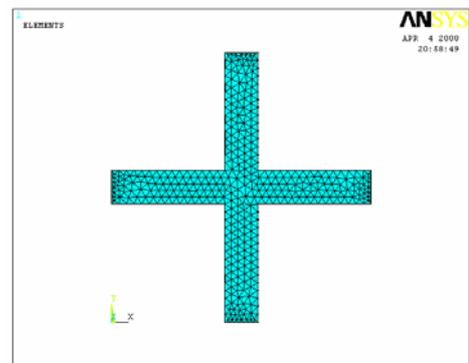
Figure (2) The FEM model of biaxial creep sample.
