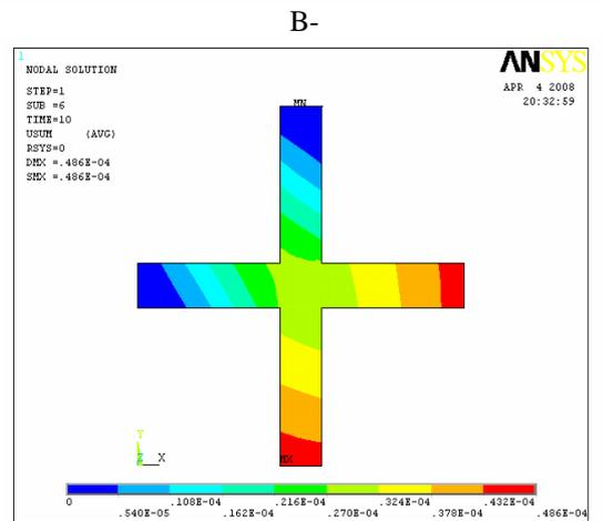
Figure (9(A,B)) FEA of deformation in the biaxial(x,y) specimen of pure low density Polyethylene.
