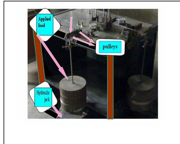
Figure (4) biaxial creep apparatus.
