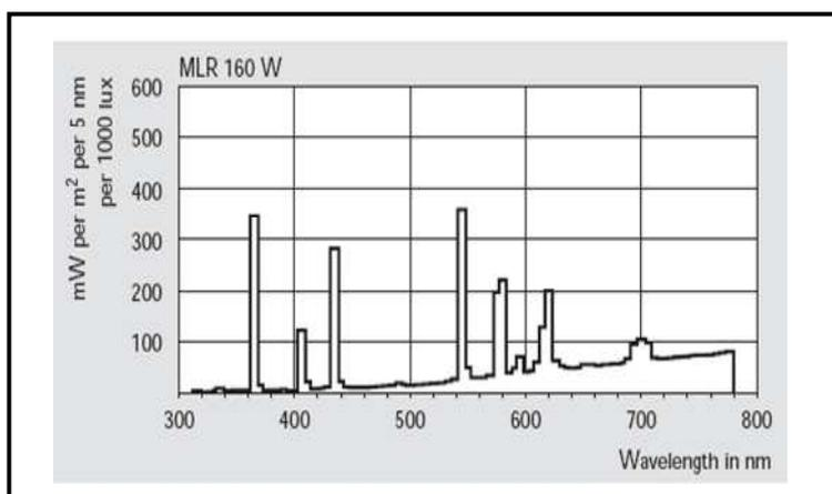
**Figure (2):- The spectrum of irradiation OSRAM lamp.**
