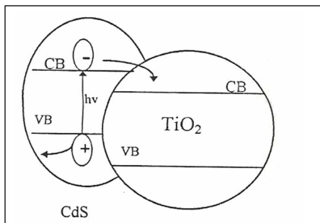
**Figure(1):- Illumination of coupled TiO<sub>2</sub>/CdS .**
