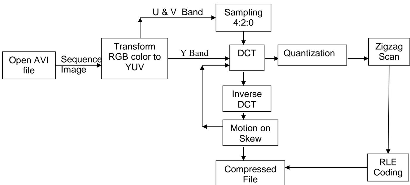
Figure (2): Block Diagram of Coder Part
