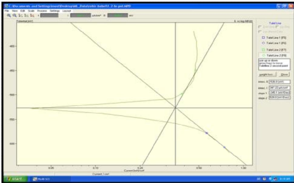
Figure ( 8 ) Show the potentiostatic curves between potential and current density for ( Cu +13wt%Al+3.8wt%Ni + 1.2wt% Fe ) alloy.
