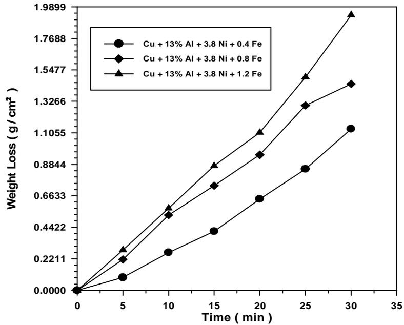
Figure ( 3 ) Shows the relation between weight loss during dry sliding with time for ( Cu +13wt%Al+3.8wt%Ni ) alloy with the effect of Fe additives
