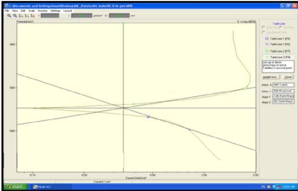
Figure ( 7 ) Show the potentiostatic curves between potential and current density for ( Cu +13wt%Al+3.8wt%Ni + 0.8wt% Fe ) alloy.
