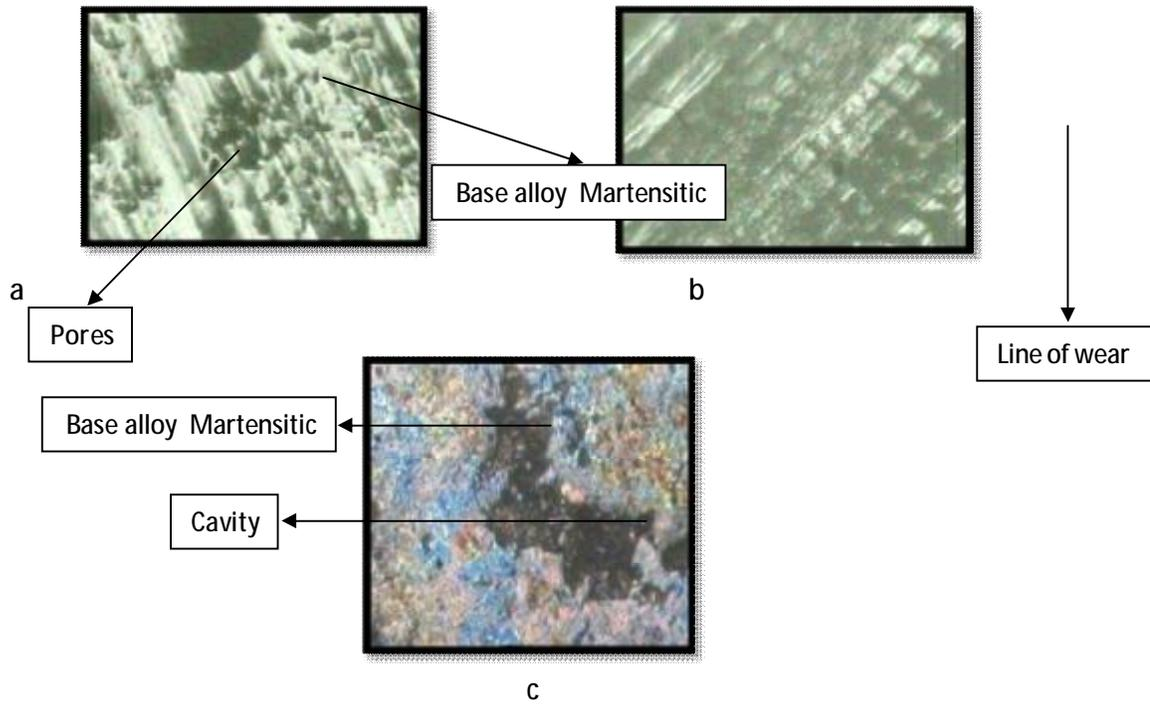
**Figure ( 12) a-Surface of ( Cu +13wt%Al+3.8wt%Ni+0.8wt% Fe ) alloy (750X) as quenched condition.**
