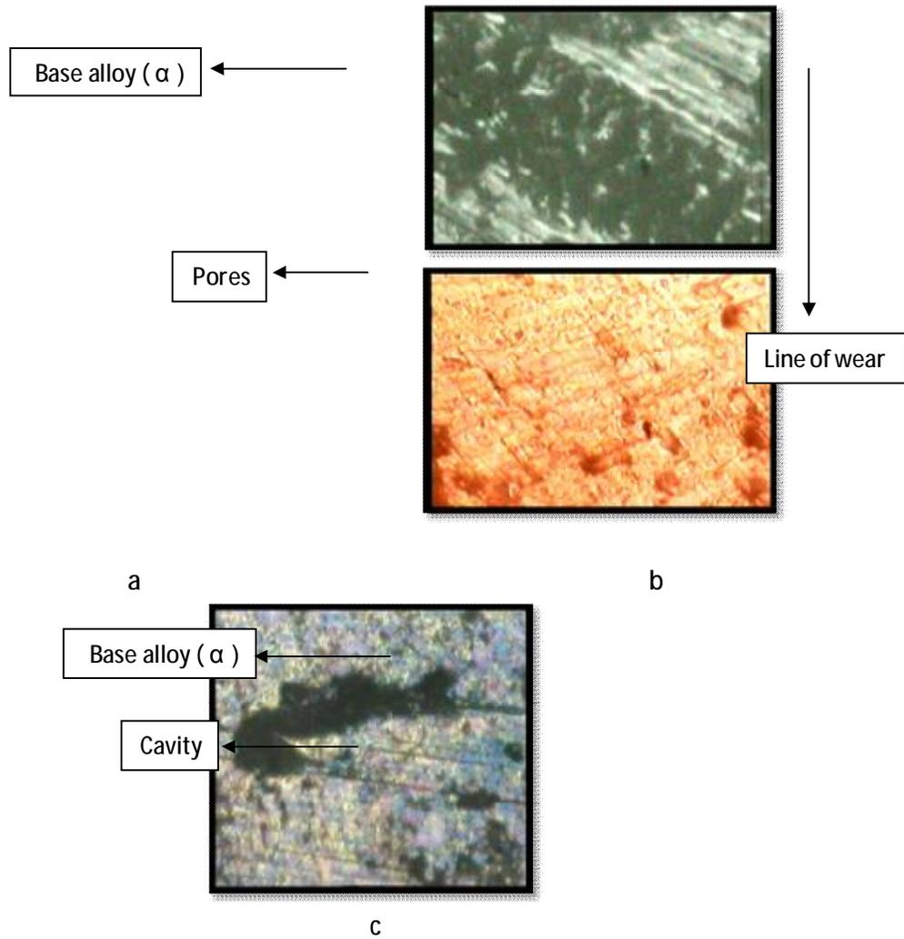
**Figure ( 9 ) a-Surface alloy in sintered case(750X ).
