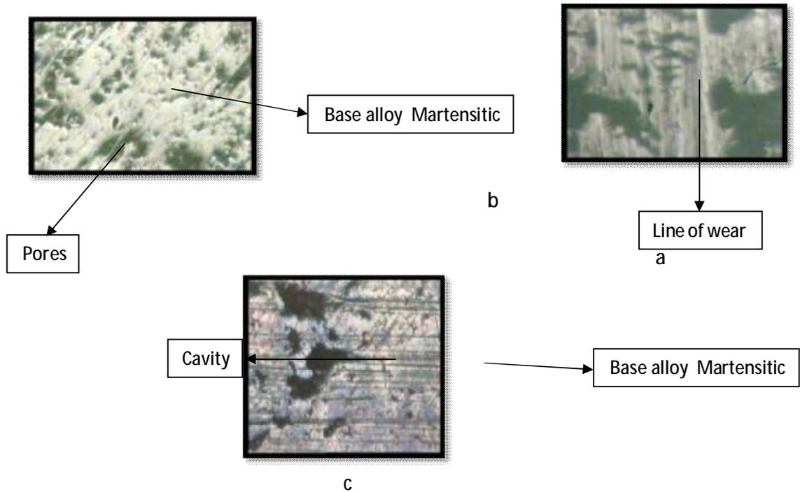
**Figure ( 13)a- Surface of ( Cu +13wt%Al+3.8wt%Ni+1.2wt% Fe ) alloy (750X) as quenched condition.**
