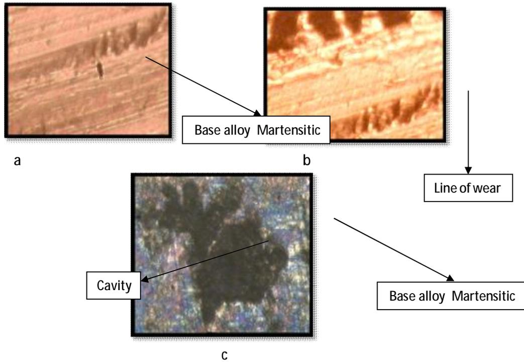
Figure ( 10 )a- Surface of alloy after Quenching in iced water (750X ).
