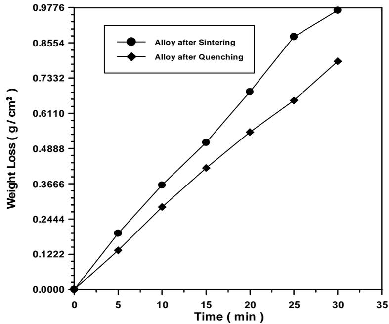
Figure ( 2 ) Shows the relation between weight loss during dry sliding with time for ( Cu +13wt%Al+3.8wt%Ni ) alloy in sintering case and after quenching in iced water.
