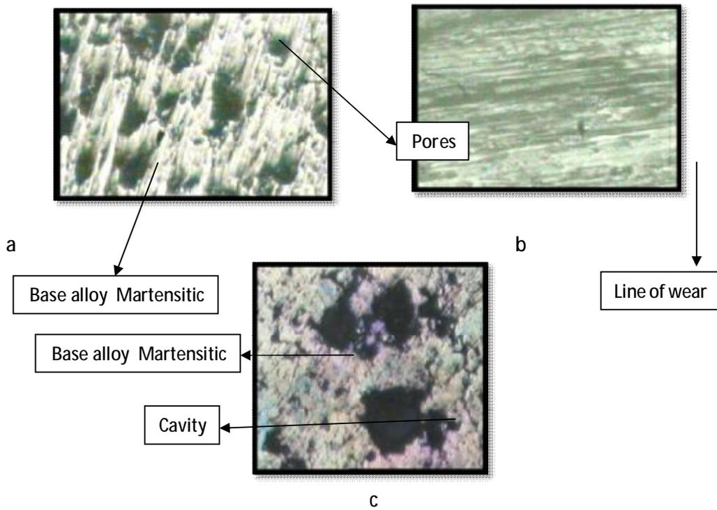
**Figure ( 11) a- Surface of ( Cu +13wt%Al+3.8wt%Ni+0.4wt% Fe ) alloy (750X) as quenched condition .**
