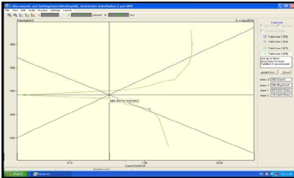
Figure ( 5 ) Show the potentiostatic curves between potential and current density for ( Cu +13wt%Al+3.8wt%Ni ) alloy after quenching in cold water.
