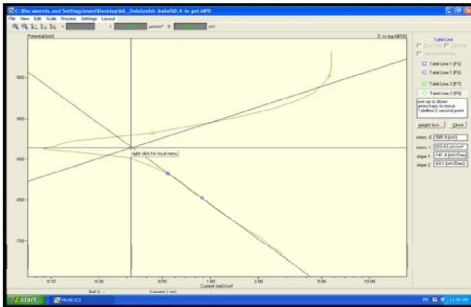
Figure ( 6 ) Show ) Show the potentiostatic curves between potential and current density for ( Cu +13wt%Al+3.8wt%Ni + 0.4wt% Fe ) alloy.
