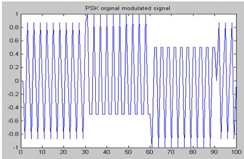
Figure 4, a) PSK original modulation signal
