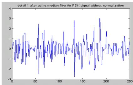
c) Detail after using median filter for FSK signal without normalization
