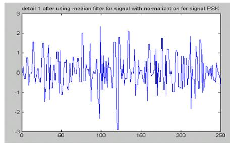
d) Detail after using median filter for PSK signal with normalization
