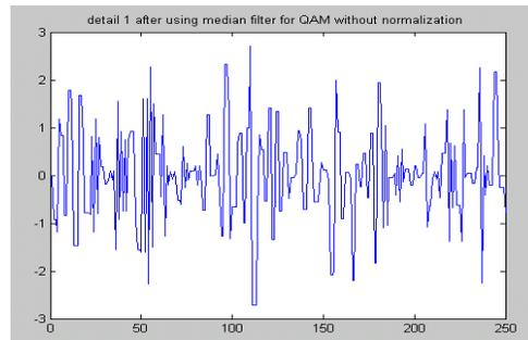
b) Detail after using median filter for QAM signal without normalization
