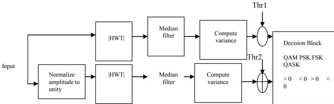
Figure 1. Block diagram of the digital modulation identifier.
