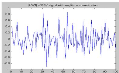
c) [HWI] of PSK signal with amplitude normalization
