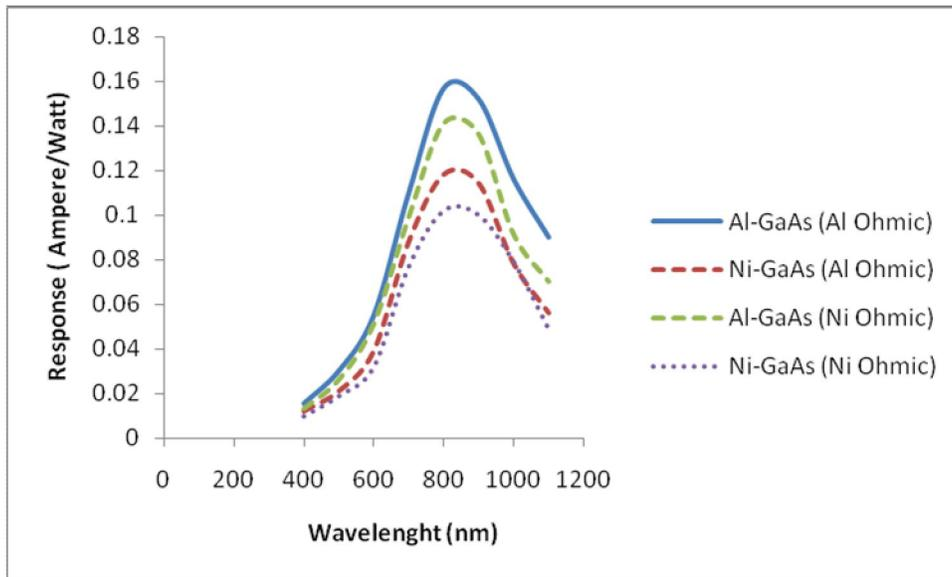
**Figure (4) Response for the four samples as a function of the wavelength**
