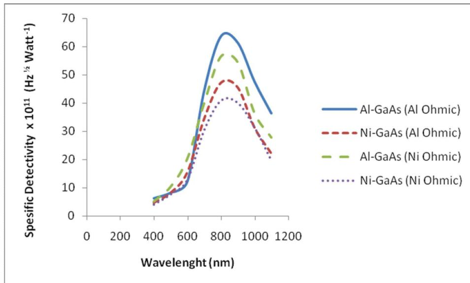
**Figure (5) specific detectivity for the four samples as a function to the wavelength**
