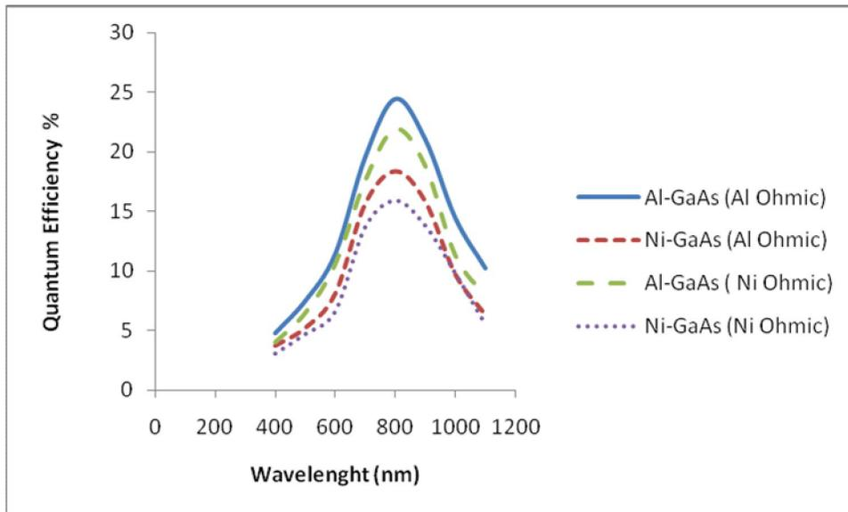
Figure (7) Quantum efficiency for the four samples as a function to the wavelength
