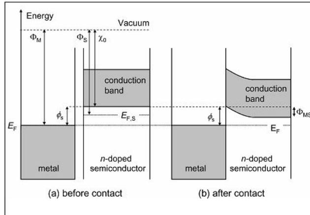
**Figure (1) Metal-semiconductor (a) before contact (b) after contact**
