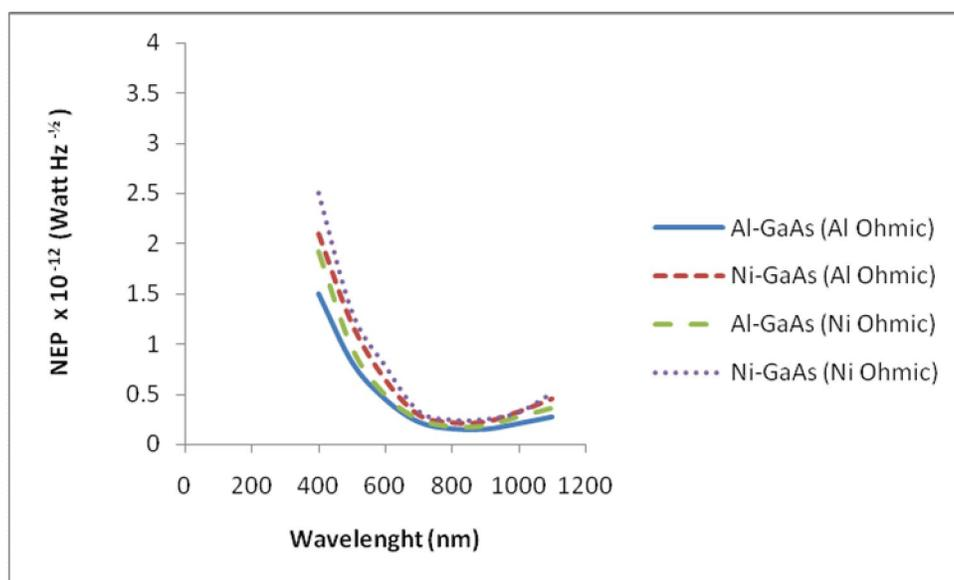
**Figure (6) Noise equivalent power for the four samples as a function to the wavelength**
