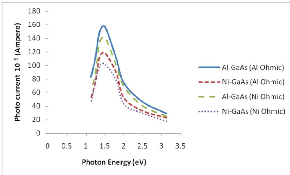
**Figure (3) Photocurrent for the four samples as a function to the photon energy**
