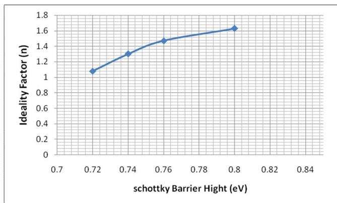
**Fig(6) shows the relation between (SBH) and (n) at room temperature**
