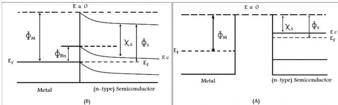
**Fig. 1: Schottky contact between metal and n- semiconductor**
