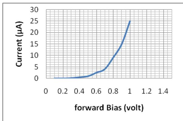
**Fig (5)Ni-GaAs (Ni Ohmic)**
