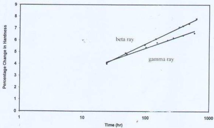
Figure.2. Semi-log graph of percentage change in hardness versus irradiation time
