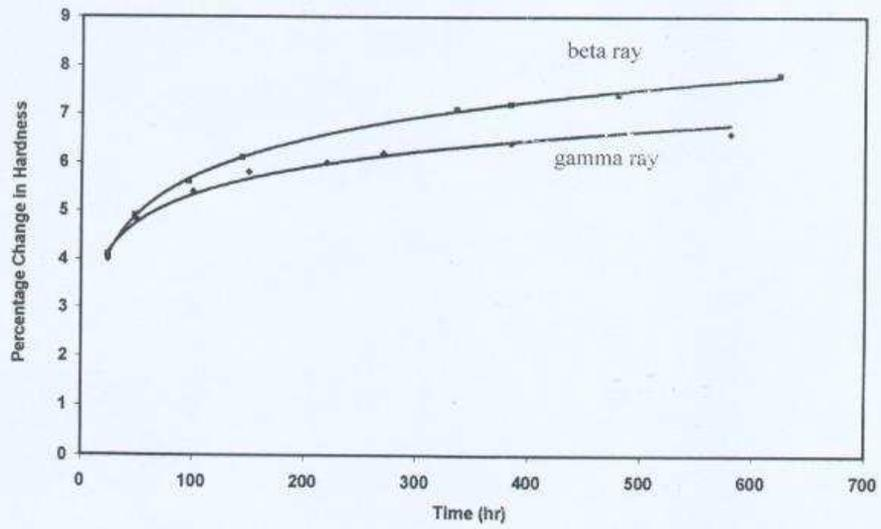
Figure.1. Percentage change in hardness as a function of irradiation time of gamma
