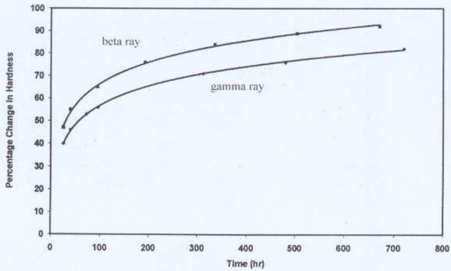
Figure.3. Percentage change in hardness as a function of irradiation time of gamma
