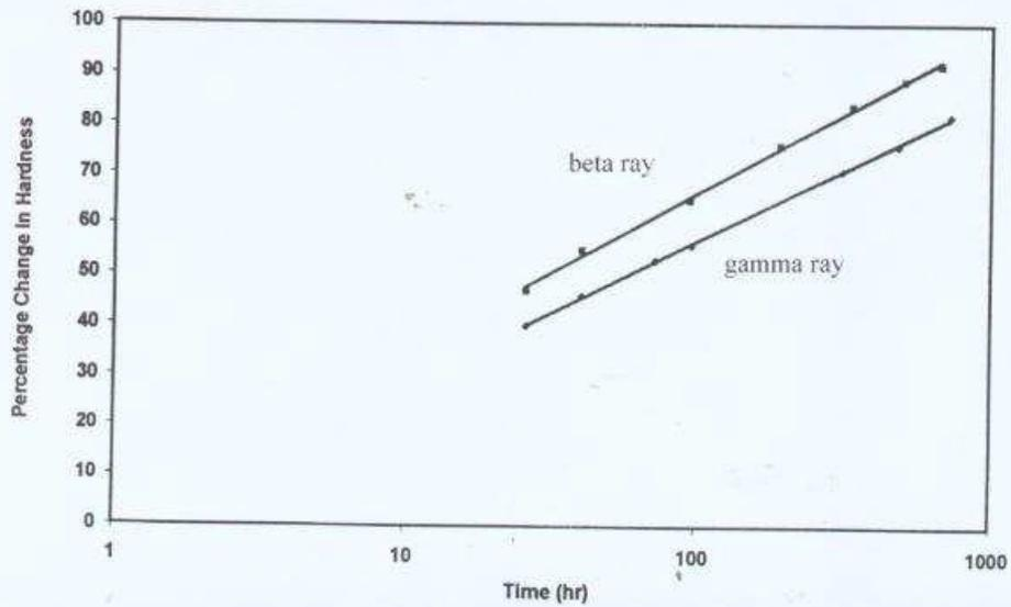
Figure.4. Semi-log graph of percentage change in hardness versus irradiation time
