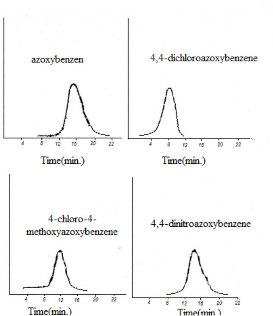
**Fig (1) HPLC chromatograms of azoxybenzene and the three derivatives, a: azoxybenzene b: 4,4-dichloroazoxybenzene, c: 4-chloro-4-methoxyazoxybenzene d: 4,4-dinitroazoxybenzene, mobile phase (80% methanol)**
