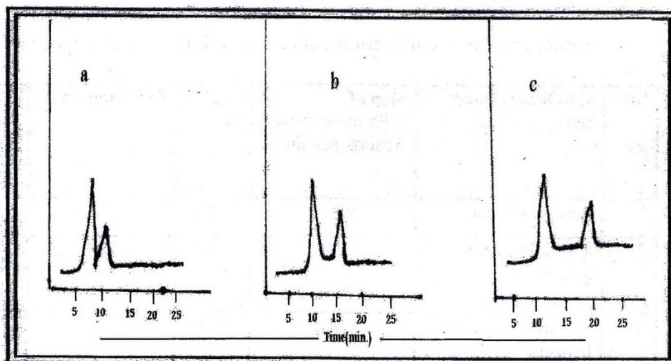
**Fig (8): Chromatograms of 4-chloro-4-methoxy azoxybenzene show the effect of methanol percentage which a: 90% v/v methanol.b:85%v/v,c: 80% v/v with a flow rate of  $1.2\text{cm}^3/\text{min}$  at  $50\text{C}^\circ$ .**
