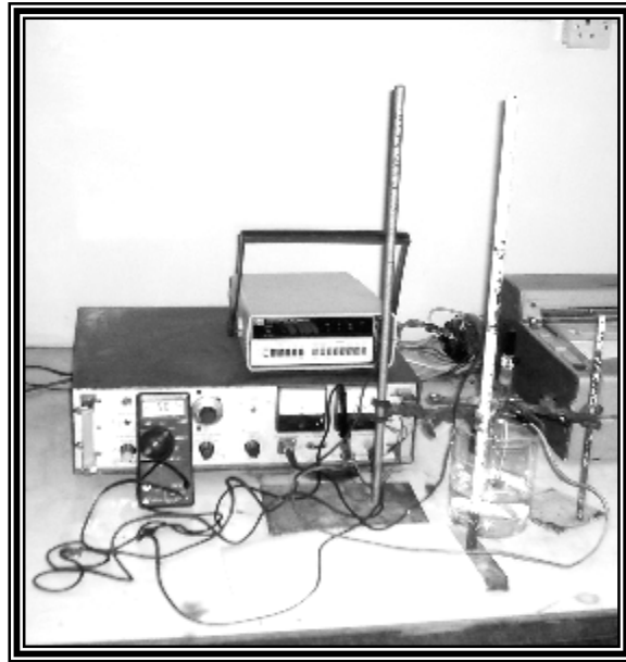
Fig. 1: Tafel extrapolation apparatus for electrochemical tests.
