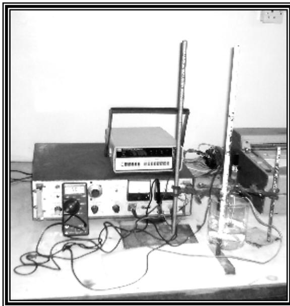
Fig. 1: Tafel extrapolation apparatus for electrochemical tests.
