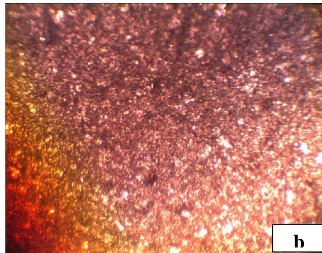
**Fig. 4: light optical micrograph for as polished aluminum reinforced by 12wt.%  $\alpha$ -Al<sub>2</sub>O<sub>3</sub> particles (a) before sintering process, (b) after sintering process Alumina particles appear darker than the aluminum matrix.**
