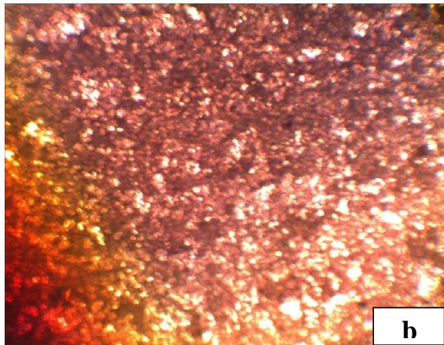
**Fig. 3: light optical micrograph for as polished aluminum reinforced by 6 wt.%  $\alpha$ -Al<sub>2</sub>O<sub>3</sub> particles (a) before sintering process, (b) after sintering process Alumina particles appear darker than the aluminum matrix.**
