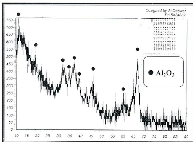
Fig. 1: Diffractograms from the surface of  $\alpha$ -(Al<sub>2</sub>O<sub>3</sub>) particles.
