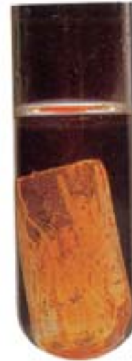
Phosphorus is a non-metallic element. It must be stored underwater (above), since it catches fire when exposed to air, forming a compound.
