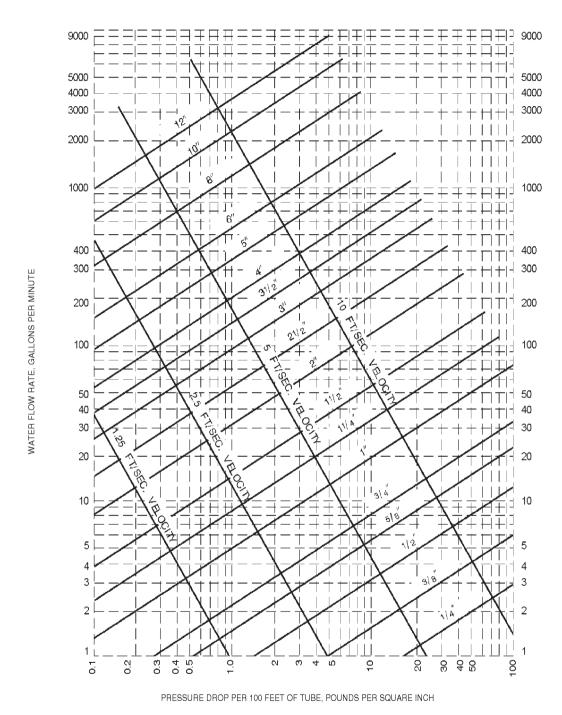
Note: Fluid velocities in excess of 5 to 8 feet/second are not usually recommended.
