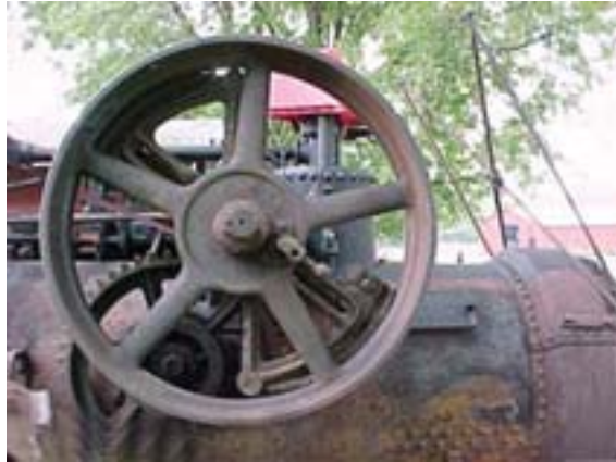
Flywheel of small steam engine.
