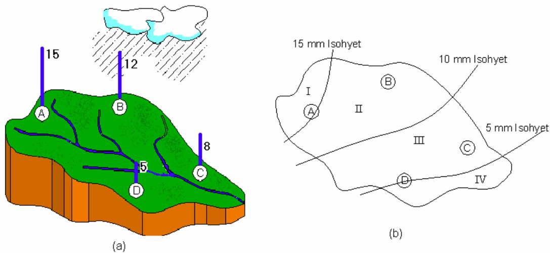
FIGURE 4. Rainfall measurement by the Isohyetal method. (a) Recorded rainfall; (b) Isohyets and the areas enclosed between two consecutive isohyets.
