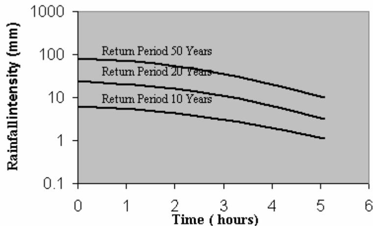
FIGURE 6. A typical rainfall intensity-duration-frequency (IDF) curve
