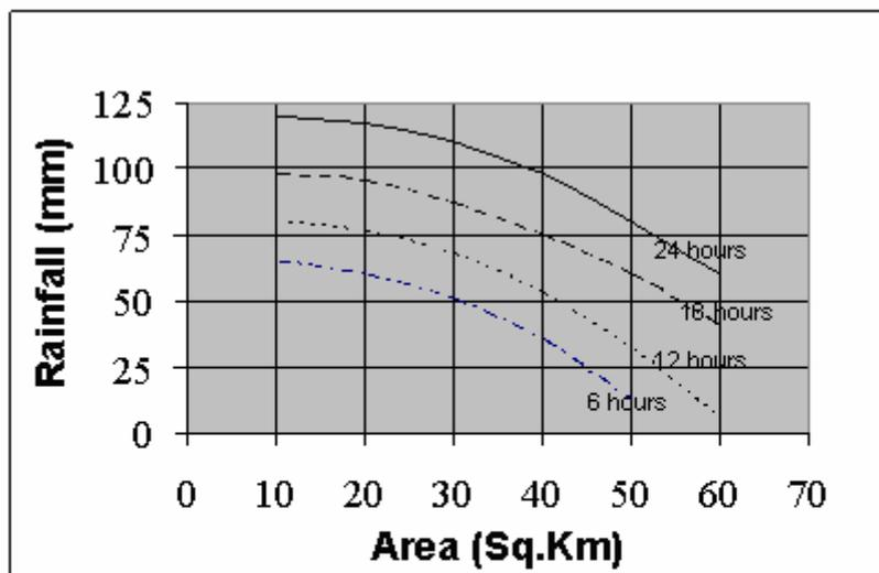
FIGURE 5. A typical Depth-Area-Duration (DAD) curve
