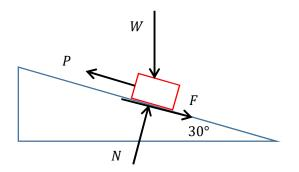
Since the reaction force (N) is normal (perpendicular) to the inclined surface and the vertical axis (y-axis) is perpendicular to the horizontal axis (x-axis), then the angle of the inclined surface with the horizontal axis ( $30^\circ$ ) is equal to the angle of the reaction force (N) with the vertical axis ( $30^\circ$ ).
