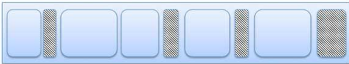
Fragmented memory before compaction
