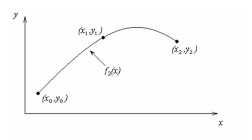
$$f_2(x) = b_0 + b_1(x - x_0) + b_2(x - x_0)(x - x_1)$$
