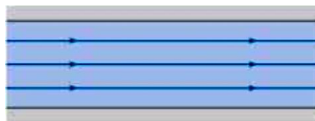
Figure 12.3 Uniform flow in a pipe
