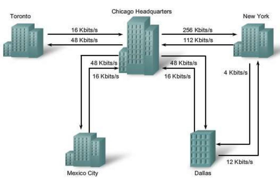
• The first thing to consider is the bandwidth requirement of each site. Working out from the headquarters, the Chicago to New York connection requires a maximum speed of 256 kb/s. Three other sites need a maximum speed of 48 kb/s connecting to the headquarters, while the connection between the New York and Dallas branch offices requires only 12 kb/s.
