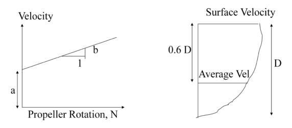
Considering the velocity profile with depth, average value of velocity can be obtained at 0.6 of the depth. i.e. V = average velocity is at about 0.6 D.
