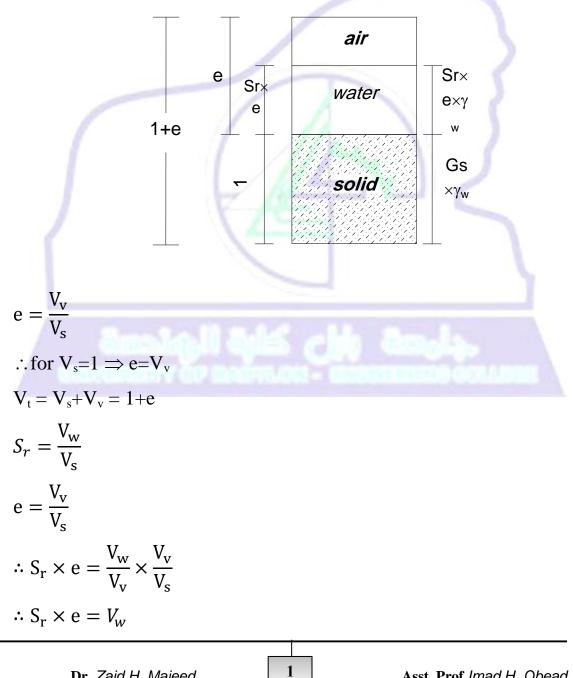
$$W_{w} = V_{w} \times \gamma_{w} = S_{r} \cdot e \cdot \gamma_{w}$$
