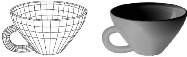
Figure 2-16 Polygon Mesh Representation and Rendering of a Teacup
