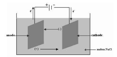
In molten sodium chloride (NaCl), there are two ions, namely, cation  $Na^+$  and anion  $Cl^-$ . At the anode, the oxidation of chloride ion takes place by depositing two electrons and forming a pure chlorine gas. At the same time, the reduction of sodium ion takes place at the cathode forming a pure sodium metal. The reactions at both electrodes are given below:
