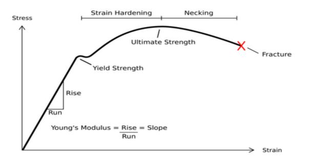
Typical stress vs. strain diagram with the various stages of deformation.
