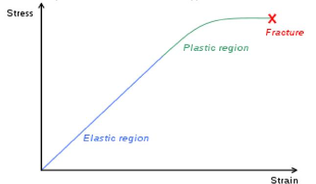
Diagram of a <u>stress-strain curve</u>, showing the relationship between stress (force applied) and strain (deformation) of a ductile metal.
