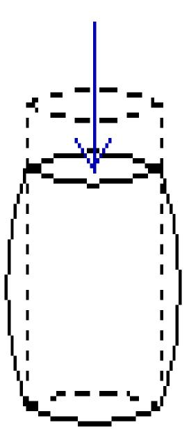
Compressive stress results in deformation which shortens the object but also expands it outwards.
