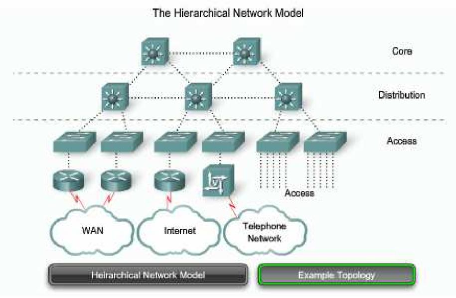
The figure represents the Hierarchical Network Model in campus environments. The Hierarchical Network Model provides a modular framework that allows flexibility in network design, and facilitates ease of implementation and troubleshooting in the infrastructure. However, it is important to understand that the network infrastructure is only the foundation to a comprehensive architecture.
