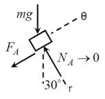
**Ex. (8):** A small vehicle enters the top *A* of the circular path with a horizontal velocity  $v_0$  and gathers speed as it moves down the path. Determine an expression for the angle  $\beta$  which locates the point where the vehicle leaves the path and becomes a projectile. Evaluate your expression for  $v_0 = 0$ . Neglect friction
