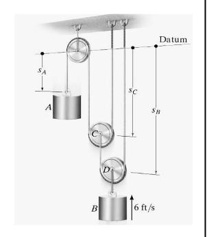
**Ex. (21):** Neglect the diameters of the small pulleys and establish the relationship between the velocity of *A* and the velocity of *B* for a given value of *y*
