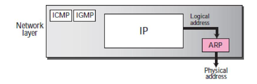
shows the position of ICMP in relation to IP and other protocols in the network layer.
