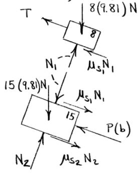
As in (a), all friction forces go to their respective maxima for impending slip.
