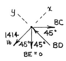
5) Determine the force in each member of the truss.
