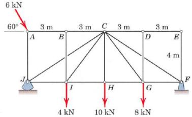
Solution From truss as a whole and  $\Sigma M_F = 0$ , J = 14.20 kN.
